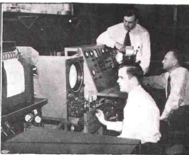
Dr. James Hillier (foreground), Dr. V. K. Zworykin (seated) and Richard L. Snyder demonstrating the recently perfected electron microscope. The picture from the facsimile printer of the instrument shows etched nickel.
